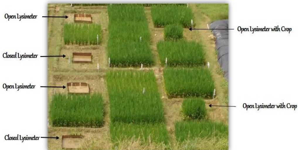
Figure 3 Lysimeters installation in field to compute deep percolation of water balance component
